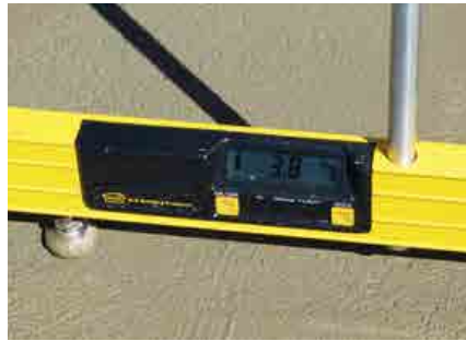
Demonstrating the reliability between a level directly on the concrete and mounted on the mag beam, a walking 300-mm (12-in.) profiler on articulating feet, and a walking profiler used on a mag screed to check the first cut.
