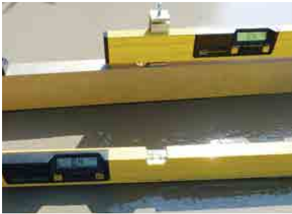
Demonstrating the reliability between a level directly on the concrete and mounted on the mag beam, a walking 300-mm (12-in.) profiler on articulating feet, and a walking profiler used on a mag screed to check the first cut.
