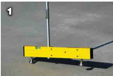
The final check of a cured surface using a walking digital profiler. Image 1 shows the lift, Image 2 illustrates the twist and rotate on one foot of the device, and Image 3 shows the final placement (i.e. both feet down) to read the slope. By twisting the knob on the handle, the articulating feet rotate to walk the measurements continuously in 300-mm (12-in.) increments. Readings or samples are taken at every other 300-mm turn—in other words, they are collected at 600-mm (24-in.) increments.
