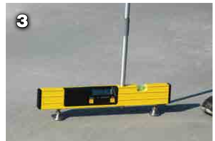
The final check of a cured surface using a walking digital profiler. Image 1 shows the lift, Image 2 illustrates the twist and rotate on one foot of the device, and Image 3 shows the final placement (i.e. both feet down) to read the slope. By twisting the knob on the handle, the articulating feet rotate to walk the measurements continuously in 300-mm (12-in.) increments. Readings or samples are taken at every other 300-mm turn—in other words, they are collected at 600-mm (24-in.) increments.
