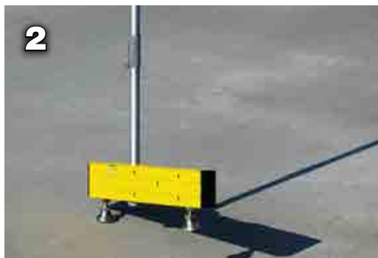
The final check of a cured surface using a walking digital profiler. Image 1 shows the lift, Image 2 illustrates the twist and rotate on one foot of the device, and Image 3 shows the final placement (i.e. both feet down) to read the slope. By twisting the knob on the handle, the articulating feet rotate to walk the measurements continuously in 300-mm (12-in.) increments. Readings or samples are taken at every other 300-mm turn—in other words, they are collected at 600-mm (24-in.) increments.
