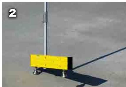
The final check of a cured surface using a walking digital profiler. Image 1 shows the lift, Image 2 illustrates the twist and rotate on one foot of the device, and Image 3 shows the final placement (i.e. both feet down) to read the slope. By twisting the knob on the handle, the articulating feet rotate to walk the measurements continuously in 300-mm (12-in.) increments. Readings or samples are taken at every other 300-mm turn—in other words, they are collected at 600-mm (24-in.) increments.
